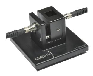
The ARCoptix CUV is our homemade cuvette holder system for transmission measurements in the near infrared. It features two fiber collimators with SMA905 connectors, a 12.5 mm wide sample port that accepts cuvette with an optical path up to 10 mm long, as well as a filter slot to avoid spurious effects (heating of the sample, extra shot noise) resulting from a too high illumination.
